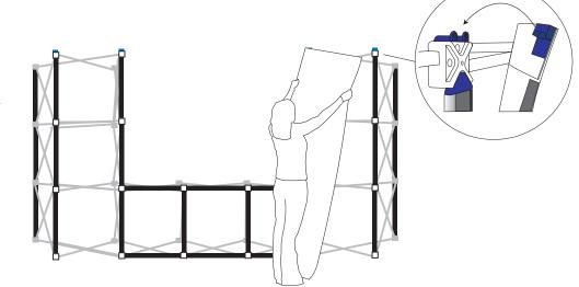
With the first two full length panels in place, use their bases to align the three short panels.
